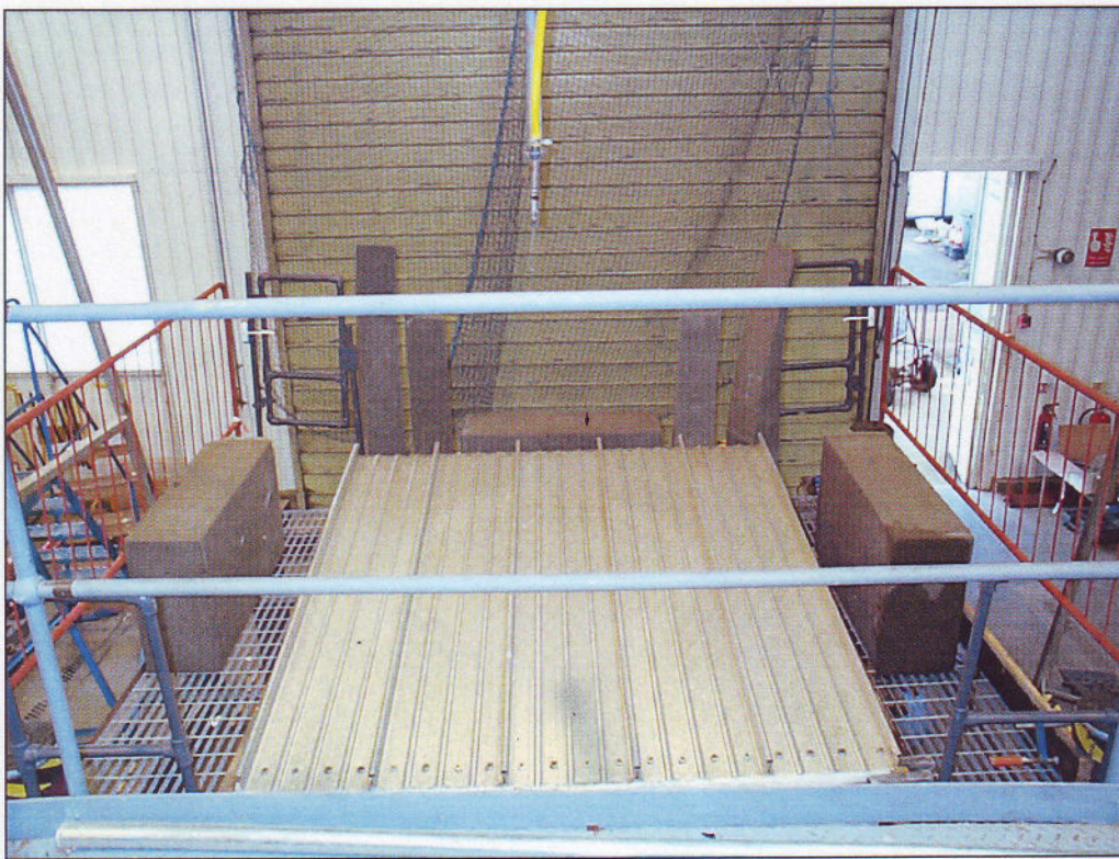
Figure 2 Roof specimen installed in test rig with nozzle used to create 'Moderate' rain
