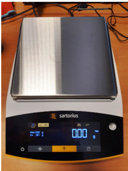
Figure 6: Precision balance used to measure the weight of the specimens.
